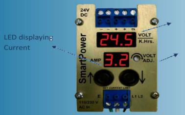
LED displaying Output Voltage
