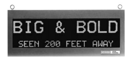
The PMD 3100 Series is a large master marquee display available in 11.5", 16.3", and 25.9" (292.1, 414, and 657.9 mm) heights and 40", 76", and 150" (1016, 1930.4, and 3810 mm) widths in a total of eight different sizes (maximum height and maximum width model is not available).
