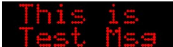
"This is" will be centered on line 1 and "Test Msg" will be centered on Line 2 of all the ToughMarquees connected on the network.
